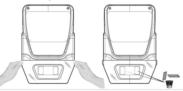
The versions with front door allow direct access to the switch miniature circuit breaker or to the top of the device installed on the DIN rail mounted inside.
